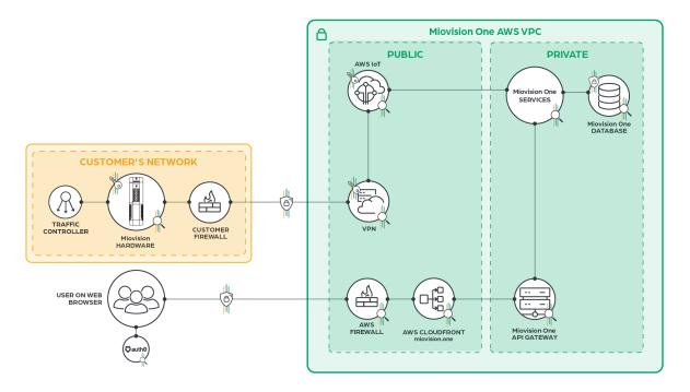
The device communicates with the Miovision One VPC via the Miovision One VPN service, over the customer network. The communication is initiated by the device and is outbound only as part of the Miovision One defense in depth approach to security.
